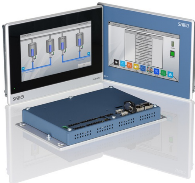
The complete assembly of the systems PLM 807-F and PLM 807-S with an application example (Source: Sabo Elektronik)
